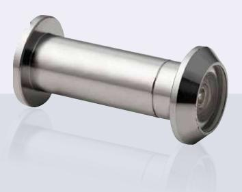
The Lockwood Security Door Viewer is constructed from solid brass and comes plated in two finishes. It features an optical glass lens providing a clear 160° angle of view. It is suited to door thicknesses of 33mm to 50mm.
