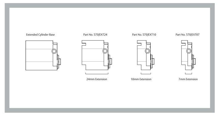
Lockwood's new Modular Cylinder Extensions provide a simple and effective method of producing an extended cylinder. The onsite flexibility of this solution will save both time and money in all applications where extended cylinders are required.
