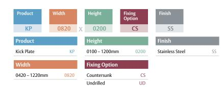
Indicate door number (if applicable), height and width of kickplates ensuring that they are within the parameters specified. Also indicate whether drilled and countersunk or undrilled kickplates are required. Pricing is determined from the closest nominal size. Kickplates are delivered labelled with sizes and door numbers (if specified).
