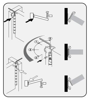
Multiple adjustment points for increasing or decreasing the spring's tension. Simple function, pull pin, turn head with allen key and replace pin. No need to remove door.
