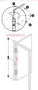
Install the spring hinge in the centre of the door between the two normal hinges.
