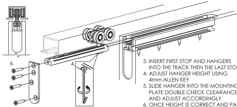
3. INSERT FIRST STOP AND HANGERS INTO THE TRACK THEN THE LAST STOP
