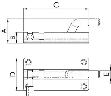
Cranked barrel bolt. The simple and popular basic door security device. The bolt is slid into the staple and the finger knob is rotated to engage in the housing slot thus locking it in position. Architectural quality.
