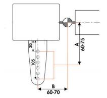
**Hinge position 2:** Fitting the DIREKT 150 to gates with hinges fixed on the middle
