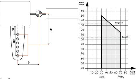
Example 1: If measure A is 105, measure B can be 30-70 mm.
