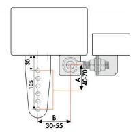
**Hinge position 3:** Fitting the DIREKT 150 to gates with adjustable hinges
