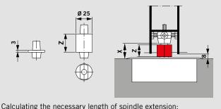
Calculating the necessary length of spindle extension:
