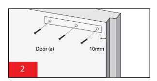
2. Install the runner plate on to door (a) positioning the plate so that the arms nylon roller runs centrally along the plate. The end of the plate closest to the leading edge of the door should be 10mm from the edge of the door.
