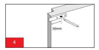
**4.** Mark out and drill the centre hole for striker plate on door (i). Hole to be on the same centre line as the runner plate fixings and 50mm from edge of door.
