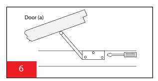
**6.** Set angle of arm if necessary by adjusting the phillips head screw contained within the end of the sequence selector mounting block.
