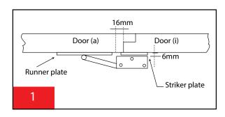
1. Install the main body of the sequence selector to the underside of the transom (door header) using the fixing screws provided.
