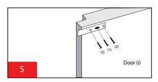
**5.** Screw striker plate to door (i) through the centre elongated fixing hole and adjust until the end clears door (a) by 3mm. Tighten screw (1) and check sequencing operation. Firmly fasten the striker plate with the remaining two screws. (2)
