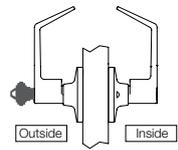
> Function: Outside lever locked and unlocked by key. Inside lever always unlocked
