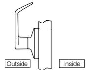
> Function: Single lever fixed. Always unlocked with no latching function.
