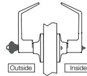
> Function: Turn/push-button locking, pushing and turning button locks outside lever requiring use of key until button is manually unlocked.
