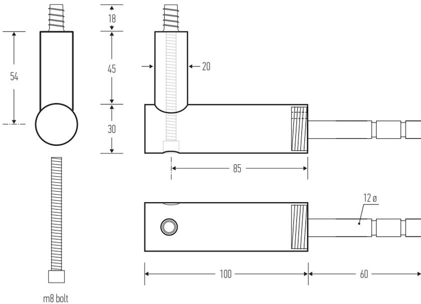
Halliday + Baillie brackets are tested in accordance with both the AS/NZS 1170.1:2002 (Structural Design Actions) standards and the International Building Code, IBC (2003) to comply with the 200lb fall ratings.
