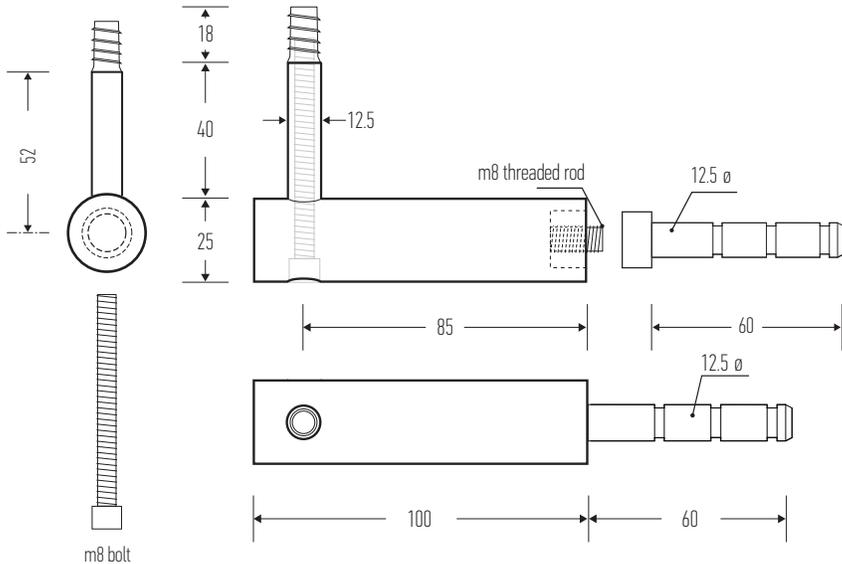
Halliday + Baillie brackets are tested in accordance with both the AS/NZS 1170.1:2002 (Structural Design Actions) standards and the International Building Code, IBC (2003) to comply with the 200lb fall rating.
