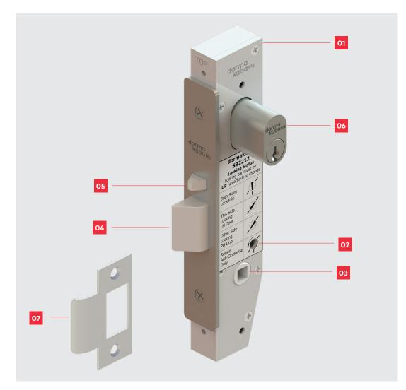
01 Zinc die cast casing 02 Lock multi-function setting 03 7.6mm split spindle hubs 04 Stainless steel latch bolt 05 Stainless steel auxiliary dead latch 06 Suitable for oval cylinder 07 Universal strike plate
