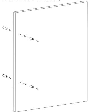
Carefully install the Entry Pull bar over the posts
