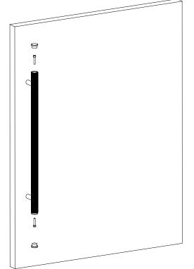
Once secured, install bar end pieces and tighten by hand
