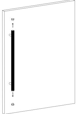
Once secured, install bar end pieces and tighten
