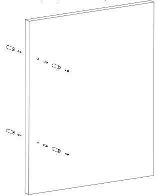
Carefully install the Entry Pull bar over the posts
