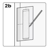
Aluminium Cutout: Match midline with template midline and position for desired backset. Mark aluminium cutout outline. Cut through aluminium.
