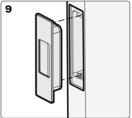
Insert end pull into cavity. Push in and down so it grips onto the bottom bracket or edge.
