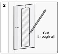
Wood Cutout: Remove middle section of flush pull template, position for desired backset and mark cutout outline. Use midline as height reference. Cut through all.
