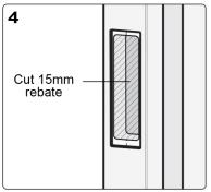
Place middle section of end pull template into rebate and mark 2nd rebate outline. Ensure it is the correct way up. Cut 15mm rebate
