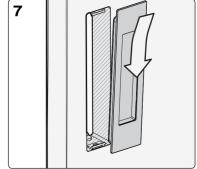
Insert flush pull into cavity. Push in and down so it grips onto the bottom bracket or edge.
