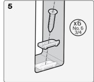
For wooden doors: install woodfix brackets at the top and bottom of cutout on both sides of the door, and on the end of the door. Six brackets total.
