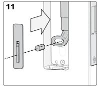
Insert spindle and emergency slide into the back of the lock slide. Choose the correct length spindle to suit your door thickness.
