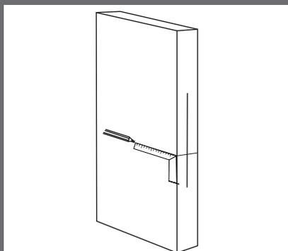
**STEP 6.** Fold the template at the desired backset between 25-70mm on the vertical line & align with the door's edge on the front of the door.
