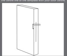
**STEP 4.** Mark a horizontal line at the bottom of the template.
