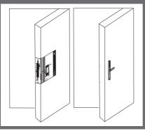
STEP 3. Mark the hole centres on the door edge for installation of the mortice lock.
