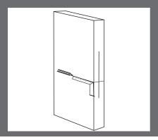
STEP 2. Measure the door thickness & mark the centre of the doors edge. Use the template to align the centre line of the template with your door centre.
