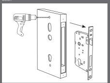
STEP 8. Drill the 14 x 19 mm holes in the edge of the door using a speed bore, set the depth to 25mm deeper then your selected backset.
