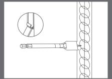
STEP 10. (A) For metal doors install a tab on the top and bottom of the mortice lock & mark the screw holes centre. Drill the 2x holes for the fixing points & install the mortice lock into the door using the tabs & screws provided.
