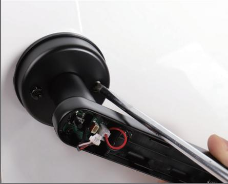
Align the square spindle & install long handle screws to mount the inside handle to the outside handle
