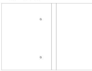
2.2. As per template, using your preferred method create a W36mm X H140mm cavity through door.
