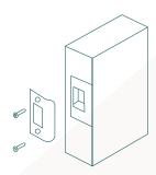
15. Close the door against the frame and mark the latch position for fitting of the striker.
