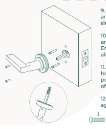
9. Unscrew the rose covers from the levers and unscrew the bolts from the threaded sleeves.
