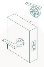
13. Insert the handle on the opposite side of the door over the spindle and tighten the long bolts through the rose into the threaded sleeves.
