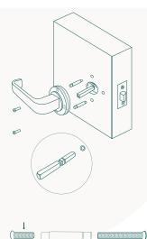
7. Remove the o-ring from the spindle. Insert the spindle into the latch so an even amount protudes on each side of the door and slide the o-ring back onto the spindle.
