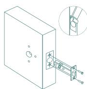
4. To change the handing of the latch, remove the outer faceplate, pull and rotate the latch tongue 180 degrees.
