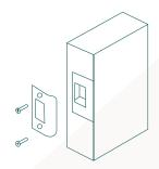
14. Close the door against the frame and mark the latch position for fitting of the striker.
