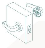
Note: The grubscrews may need a re-tighten after a bedding-in period. We recommend medium strength thread-lock to be used. 11. Slide the handle on the opposite side of the door over the spindle and tighten the long bolts through into the rose.
