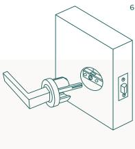
Insert handle 'A' in the 48mm hole with the spindle and rapidFIT attached and press against the door. Ensure the grooved side of the spindle is aligned with the grubscrews on the handle
