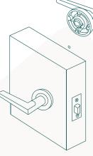
13. Insert the handle on the opposite side of the door over the spindle and tighten the long bolts through the rose into the threaded sleeves.
