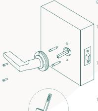
Unscrew the rose covers from the levers and unscrew the bolts from the threaded sleeves.
