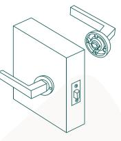
Note: The grubscrews may need a re-tighten after a bedding period. We recommend medium strength thread-lock to bed used.
