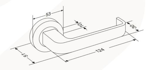
Note: Measurements are in mm
